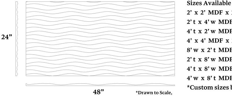
2' x 2' MDF x 3/4" d 2' t x 4' w MDF x 3/4" d 4' t x 2' w MDF x 3/4" d 4' x 4' MDF x 3/4" d 8' w x 2' t MDF x 3/4" d 2' t x 8' w MDF x 3/4" d 4' t x 8' w MDF x 3/4" d 4' w x 8' t MDF x 3/4" d \*Custom sizes by request
